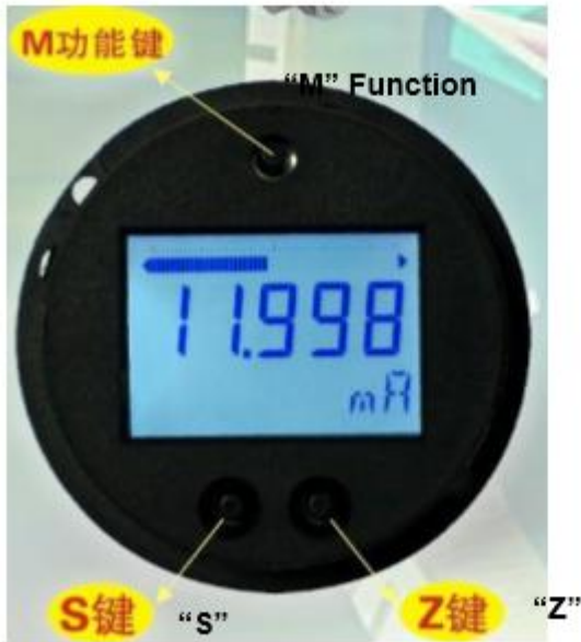
"M"- Function key, "S"- Span adjust key, "Z"- Zero adjust key.
